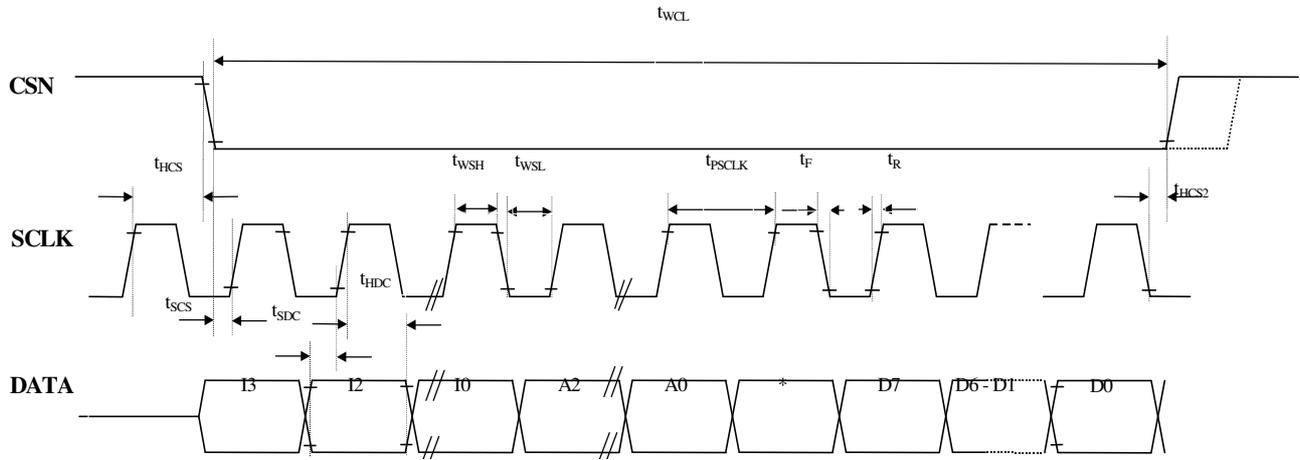
☒ 4 Serial Interface Timing < WRITE >
