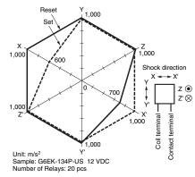
Test Conditions: Shock is applied in ±X, ±Y, and ±Z directions three times each with and without energizing the Relays to check the number of contact malfunction.
