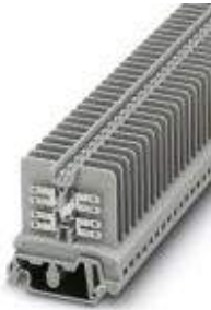
Feed-through terminal block, Connection method: Slip-on connection, Cross section: 0.5 mm 2 - 6 mm 2 , AWG: 20 - 10, Width: 6.2 mm, Color: gray, Mounting type: NS 35/7.5, NS 35/15
