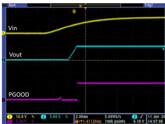
Figure 22. Power Up and PGOOD, No Load
