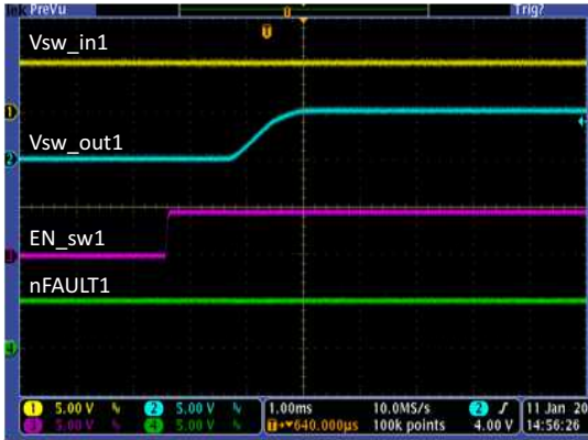
Figure 24. Power Switch1 Turn On Delay and Rise Time
