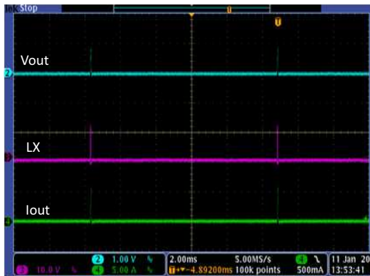
Figure 20. Buck Hiccup Response to Hard-Short Circuit
