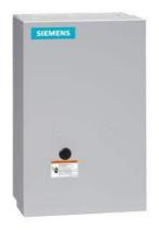
Non-reversing NEMA contactor, Size 1, Three phase full voltage, Contactor amp rating 27A, 3 wire (NO aux included), 240V 50Hz / 277V 60Hz coil, Non-combination type, Enclosure NEMA type 1, Indoor general purpose use, Extra-wide enclosure
