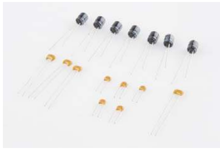
Electrolytic capacitors (top), ceramic capacitors (bottom).
