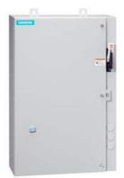
Non-reversing motor starter Size 2 1/2 Three phase full voltage Solid-state overload relay OLRelay amp range 25-100A 190-220/220-240V 50/60HZ coil Combination type 100A fusible disconnect 100A/250V fuse clip Enclosure NEMA type 4/12 Water/dust tight weather proof Standard width enclosure
