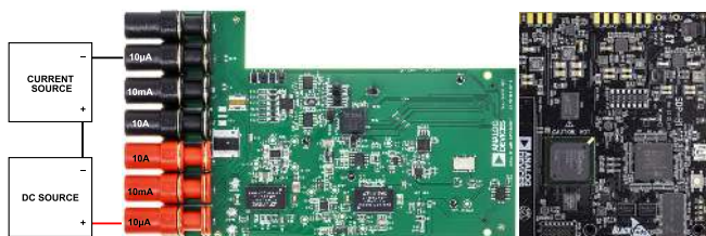
Figure 2. Simplified Evaluation Test Setup, 10 \mu A Range
