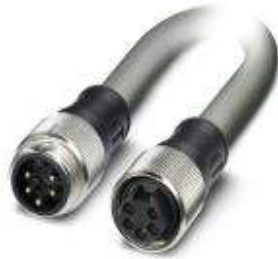
Bus system cable, DeviceNet, 5-position, PVC, Gray RAL 7001, Plug straight 7/8"-16UNF, on Socket straight 7/8"-16UNF, Cable length: 10 m
