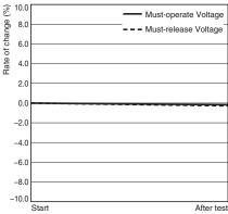
Characteristics were measured after applying vibration at a frequency of 5 to 200 to 5 Hz, acceleration of 44.1 m/s $^2$  to the test piece (not energized) for 2 hours
