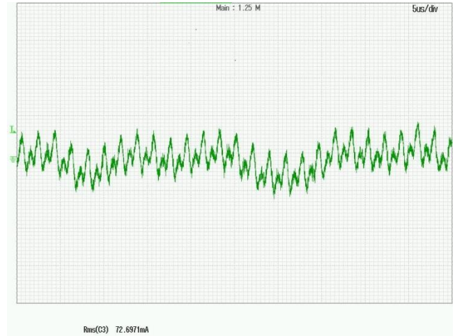
Figure 9: Input Terminal Ripple Current, i_c , at max output current and nominal input voltage with 12\mu\text{H} source impedance and 100\mu\text{F} electrolytic capacitor (200 mA/div, 5us/div).
