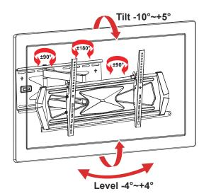
Adjust to the desired position by tilting -10°~+5°, swiveling -90°~+90°, -180°~+180°, -90°~+90° at three pivot points, and by leveling -4°~+4°.
