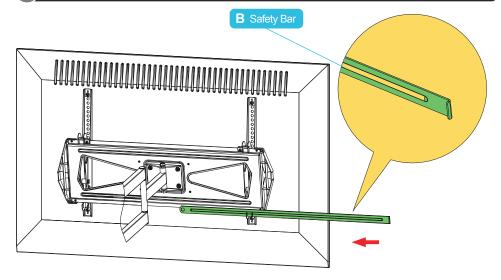
Insert the safety bar onto the rail (at the bottom of the wall plate) to secure.
