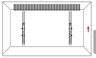
According to the direction indicator arrows on the adapter brackets, make sure the adapter brackets are installed in the correct direction.
