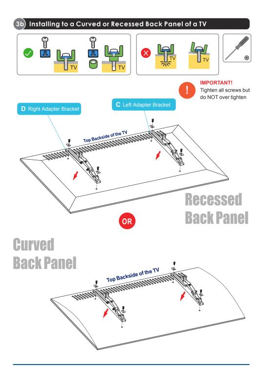
Choose the appropriate screws, washers, and spacers (if necessary) according to the type of your TV and attach adapter brackets (C and D) to the back of the TV using a Phillips screwdriver.
