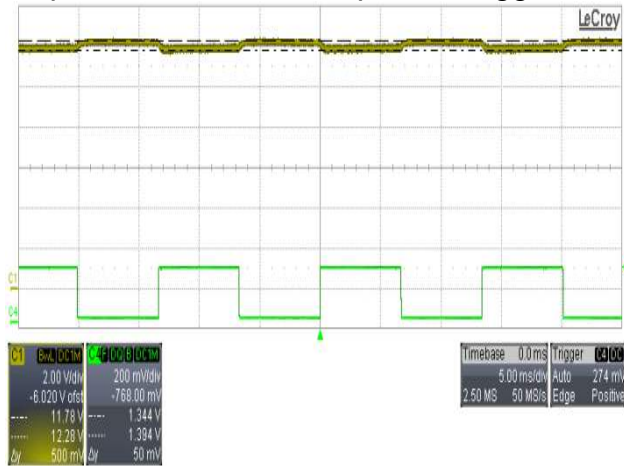
Figure 24 – Transient Response, 115 VAC, 5% \leftrightarrow 55% Step Load. Upper: V_{OUT} , 2 V / div. Lower: I_{OUT} , 1 A / div., 5 ms / div.
