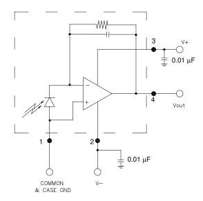
Note: Components shown outside the dashed area are external to the device, and must be supplied by the user.
