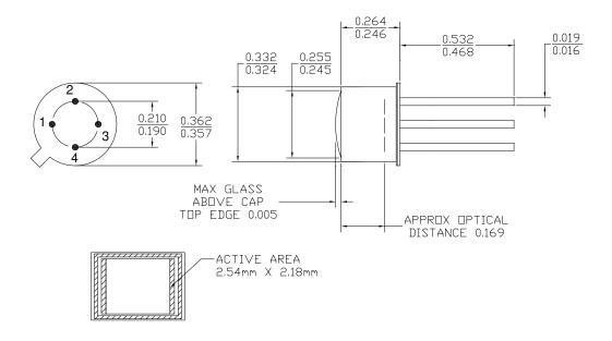
> Soldering Conditions: 260°C 1/16 inch away from case for 3 seconds max.
