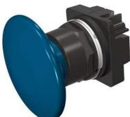
30mm BlackMax, Epoxy Coated Corrosion Resistant Metal Operator, Round Push-Pull Operator Non-Illuminated Mushroom Head Cap Large 2 1/2" (63.5 mm) Plastic, Blue 3 Position Momentary UL Listed, CSA Certified NEMA 1,3,3R,4,4X,12,13 & Automotive Standards
