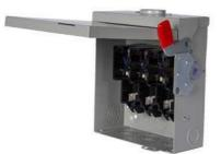
Siemens Low Voltage Circuit Protection General Duty Safety Switches. Type: ENCLOSED, SAFETY SWITCH Std: UL V. Rating: 240V A. Rating: 100A Wattage: 4W No. Of Poles: 3P F. Rating: 60Hz Action: SINGLE THROW Material: STEEL Enclosure: TYPE 1. 2-3 point mounting holes. O. Cycles: 10000 O. Temperature: (-20F-120F) AMBIENT TEMPERATURE Environmental Conditions: INDOOR
