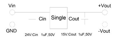
To make sure the product work at perfect operation status with full loading external capacitor is necessary and it is recommended to use high frequency low resistance electrolytic capacitor.
