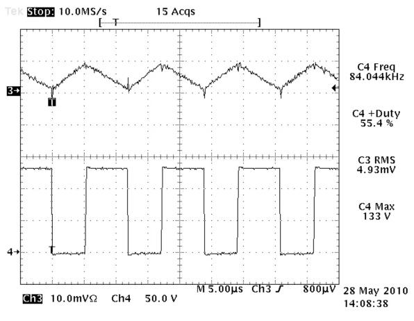
Input Voltage = 110VAC CH3: LED Current, 10mV $\Omega$  = 100mA/div CH4: MOSFET drain voltage, 50V/div Frequency = 84kHz, positive duty cycle = 55.4%
