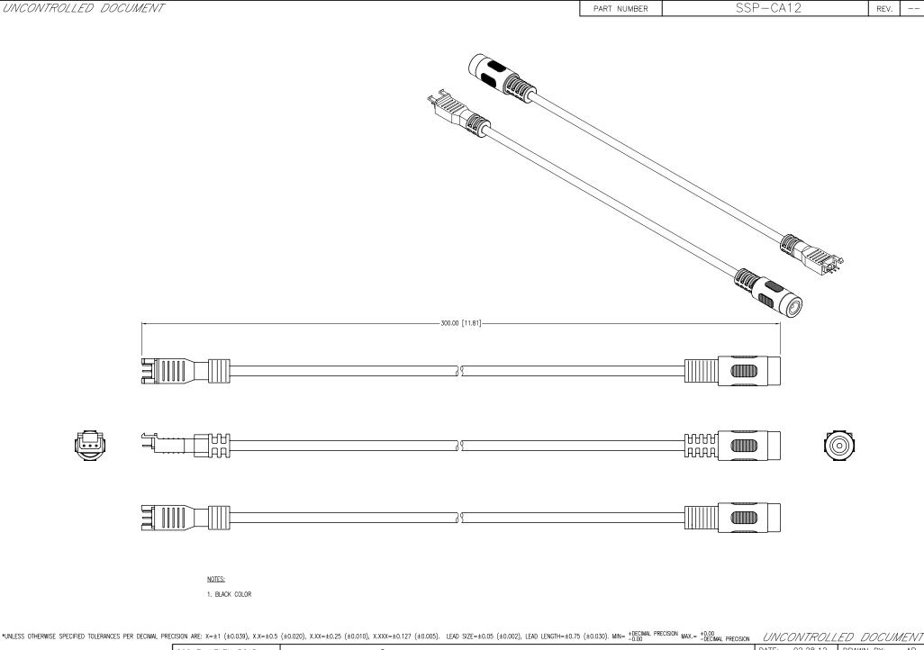
DATE: 02.28.12 DRAWN BY: AΒ 290 E. HELEN ROAD SUNBRITE 12" DIMMER SWITCH POWERLINE CONNECTION CABLE FOR MODULAR LED LIGHT BAR. PALATINE, IL 60067-6976 PAGE: 1 OF 1 CHKD BY: KF \*\*THE SPECIFICATIONS MAY CHANGE AT ANY TIME WITHOUT NOTICE DUE TO NEW MATERIALS OR PRODUCT IMPROVEMENT.\*\* PHONE: +1.847.359.2790 CONFIDENTIAL INFORMATION
