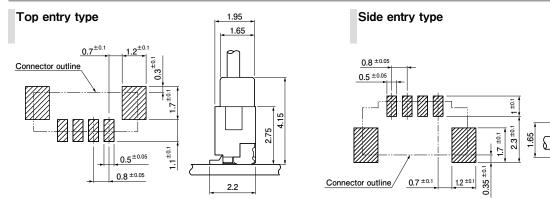
Note: 1. The above figure is the figure viewed from the connector mounting side.
