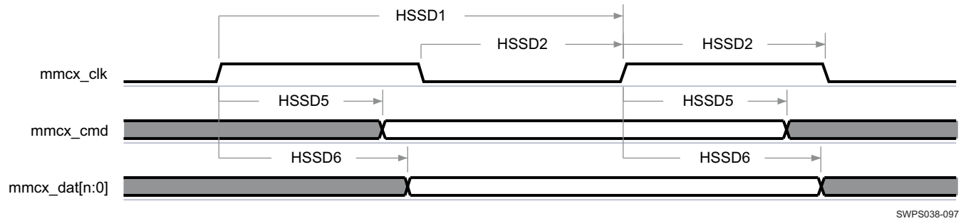
Figure 6-74. MMC2 and MMC3 Interfaces—High-Speed SDIO Mode—Data/Command Transmit (1)
