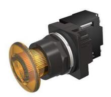
30mm BlackMax, Epoxy Coated Corrosion Resistant Complete Metal Unit Illuminated Push-Pull Operator Full Voltage, 24V AC/DC Incandescent Lamp Mushroom Head Cap Small 1 3/4" (44.5 mm) Plastic, Amber 3 Position Pull-Momentary/Push-Maintained UL Listed, CSA Certified NEMA 1,3,3R,4,4X,12,13 & Automotive Standards
