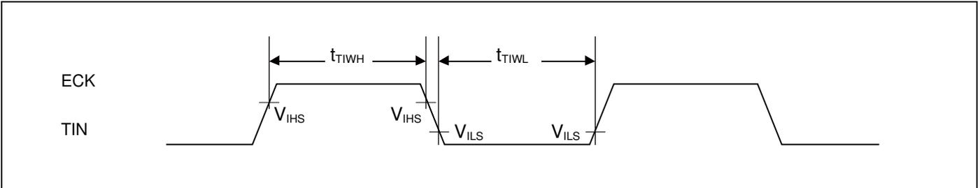
**Trigger input timing**
