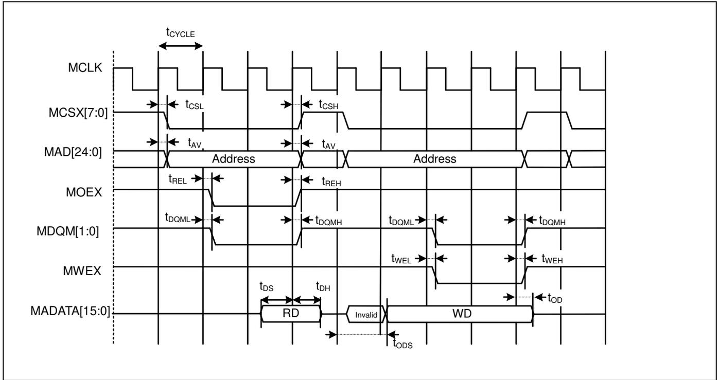
**Multiplexed Bus Access Asynchronous SRAM Mode**
