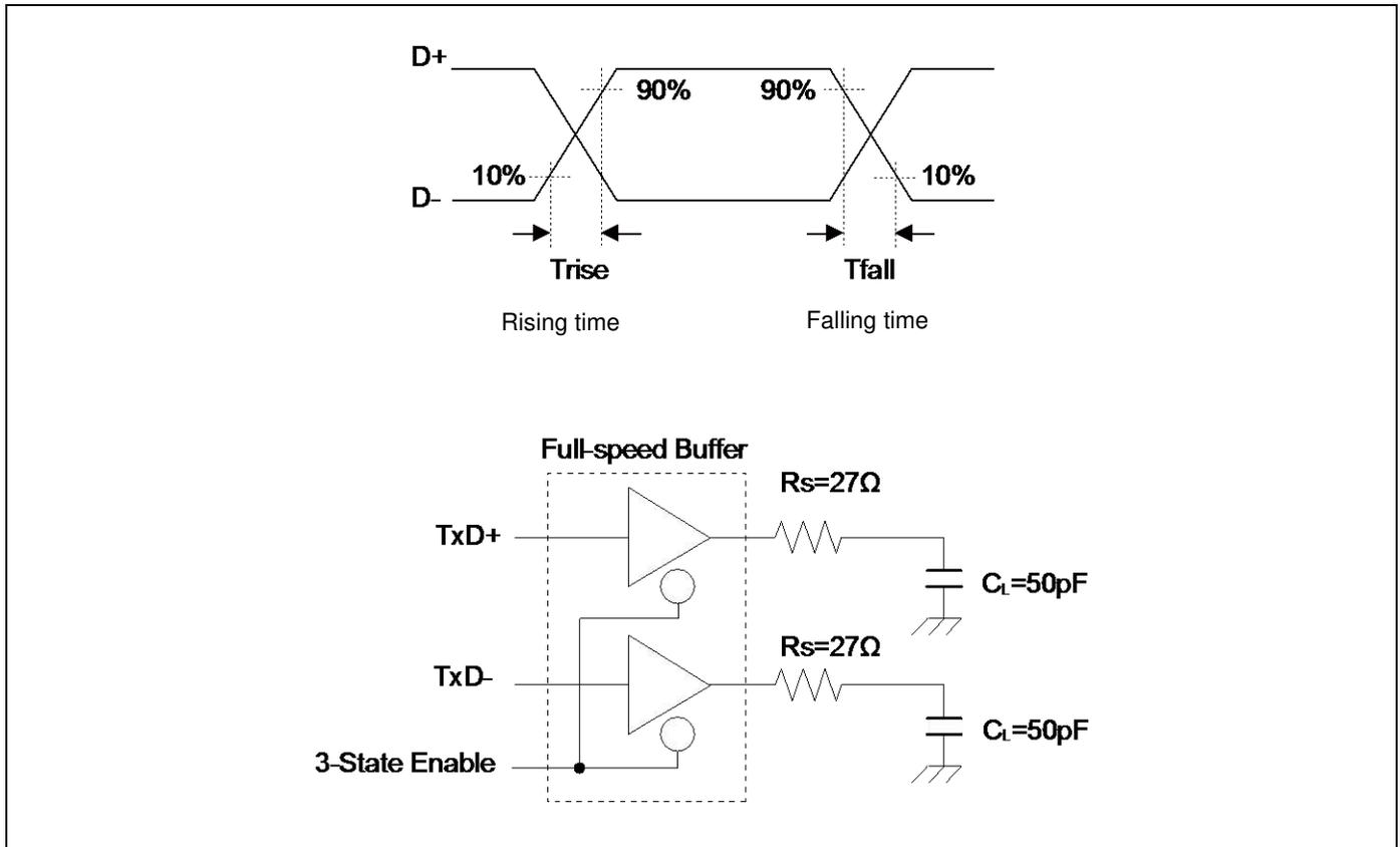
\*6: USB Full-speed connection is performed via twist pair cable shield with  $90\Omega \pm 15\%$  characteristic impedance (Differential Mode). USB standard defines that output impedance of USB driver must be in range from  $28\Omega$  to  $44\Omega$ . So, discrete series resistor ( $R_s$ ) addition is defined in order to satisfy the above definition and keep balance. When using this USB I/O, use it with  $25\Omega$  to  $30\Omega$  (recommendation value  $27\Omega$ ) series resistor  $R_s$ .
