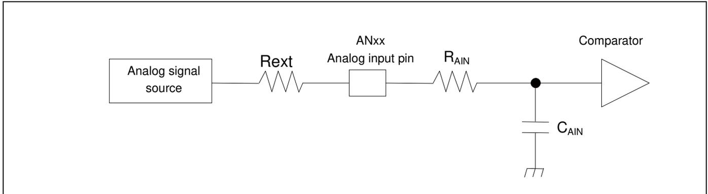
$$\text{(Equation 1) } T_S \geq (R_{AIN} + R_{ext}) \times C_{AIN} \times 9$$
