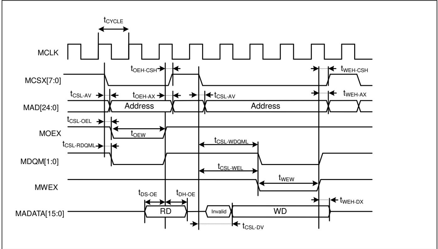
**Separate Bus Access Synchronous SRAM Mode**
