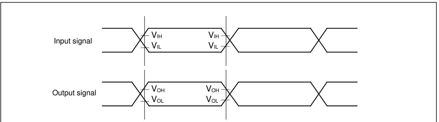
**Separate Bus Access Asynchronous SRAM Mode**
