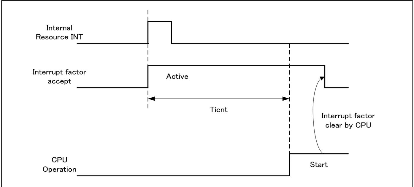
\*: Internal resource interrupt is not included in return factor by the kind of Low-Power consumption mode.
