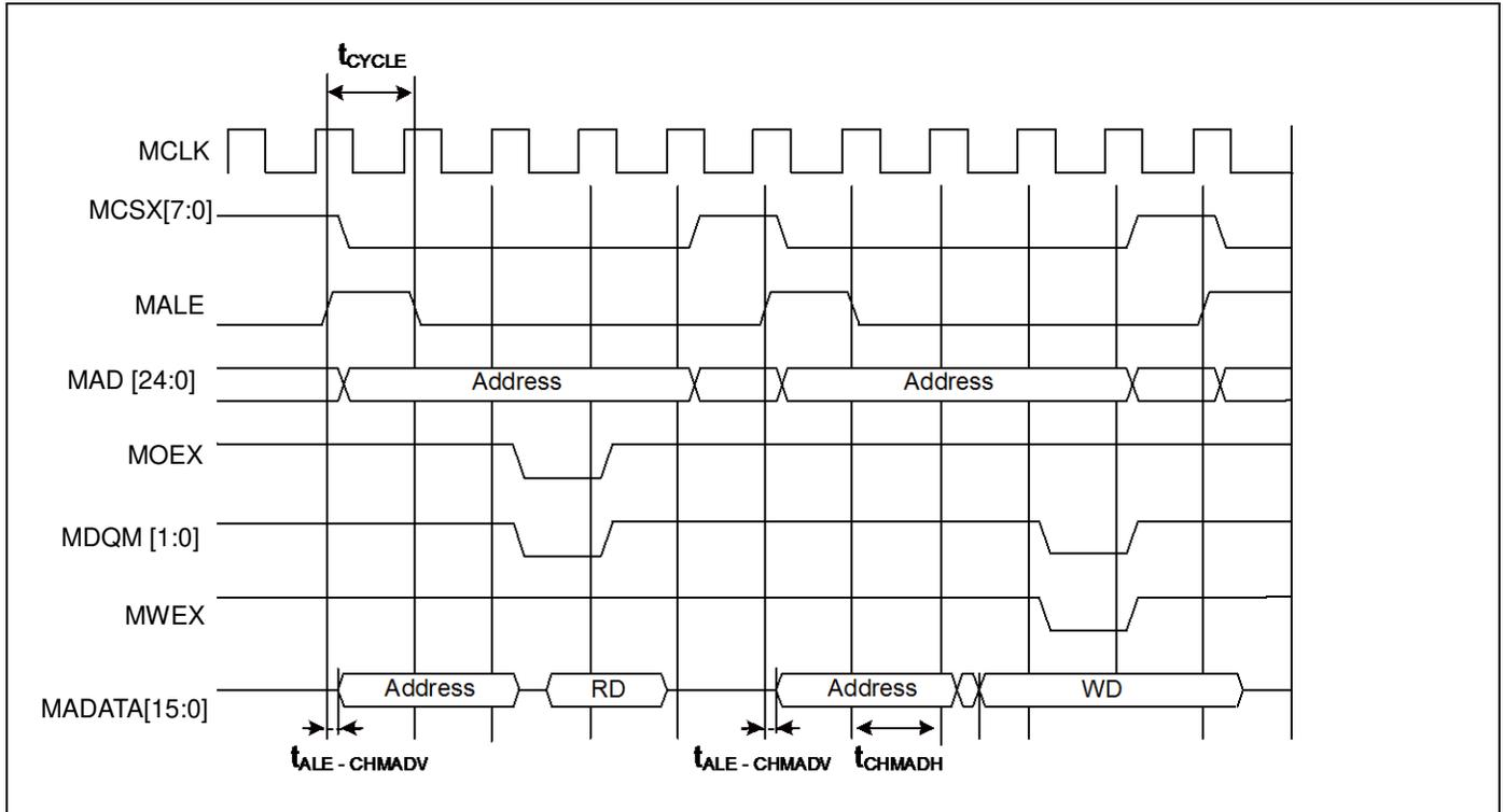
**Multiplexed Bus Access Synchronous SRAM Mode**
