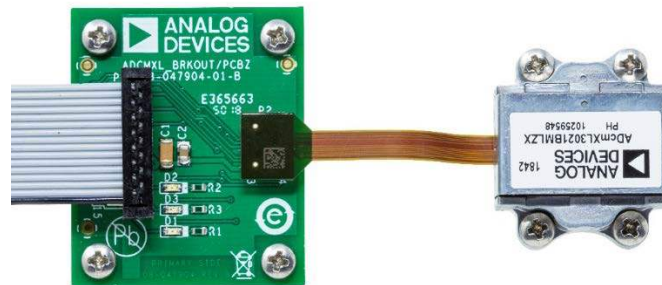
Figure 10 ADcmXL module connected to the ADCMXL_BRKOUT/PCBZ, note the direction of the ADcmXL module with respect to the board.
