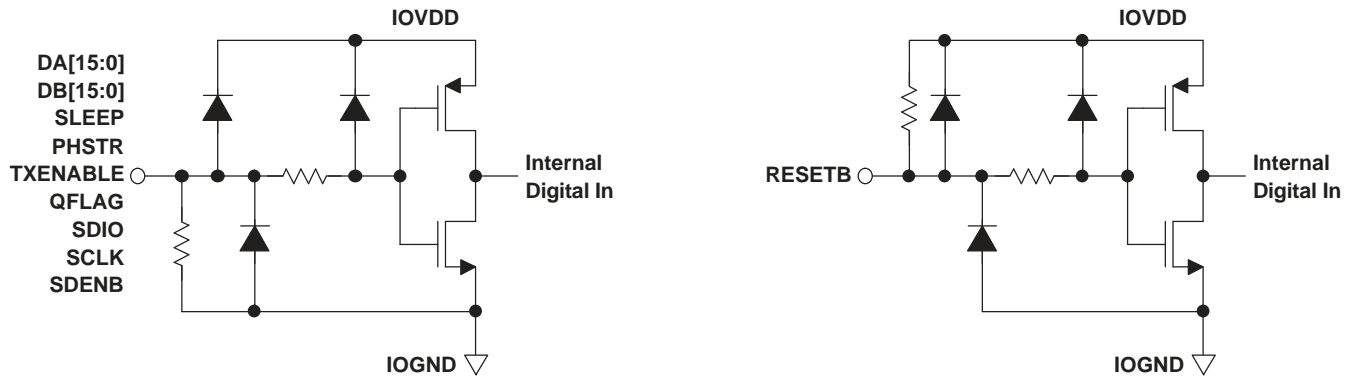
Figure 63. CMOS/TTL Digital Equivalent Input
