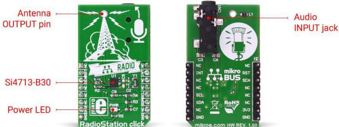
The click is designed for communication over the I2C/2-wire control interface. When selecting 2-wire mode, SCLK pin should stay at a HIGH logic level during the rising edge on the RST pin, and stay HIGH until after the first start condition. Also, a start condition must not occur within 300nS before the rising edge on the RST pin. The 2-wire bus mode uses only the SCL and SDA pins for communication.
