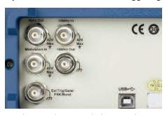
Use the external 10 MHz clock input and output to synchronize your signals to a master time base. The Sync output generates a TTL pulse for synchronization to a channel's frequency. An external trigger BNC connector is also available for inputting or generating a trigger signal.
