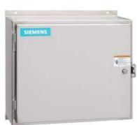
Mechanically held lighting contactor, Contactor amp rating 60Amp 0NC \_ 9NO poles, 24VAC 60HZ coil, Non-combination type, Enclosure NEMA type 12, Dust/drip proof for indoors
