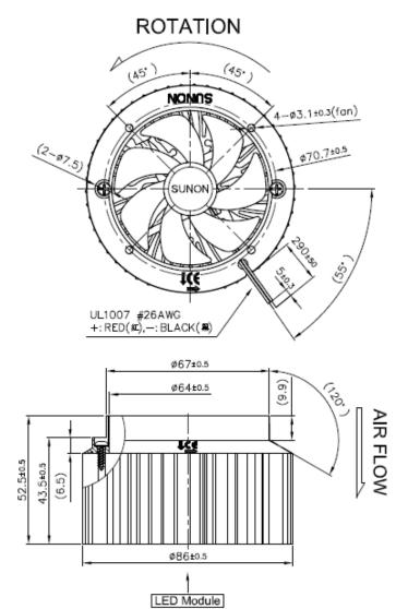
Assembly direction of customer's LED Module
