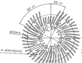
4-ø2.6±0.3 - Nmber 3 or 4 For LED Module Assembly Screw torque max 12kgf.cm
