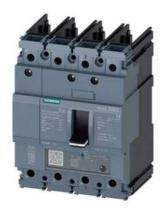
circuit breaker 3VA5 UL frame 125 breaking capacity class H 65kA @ 480V 4-pole, line protection TM230, FTAM, In=100A overload protection Ir=100A fixed short-circuit protection Ii=5...10 x In N conductor unprotected without connection
