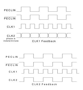
Using CLK1 as feedback will always result in synchronized rising edges between PECLIN and CLK1 if CLK1 is used as feedback. CLK2 could be a falling edge compared to PECLIN. Therefore, wherever possible it is recommended to use CLK2 for feedback, which will synchronize the rising edges of all three clocks.
