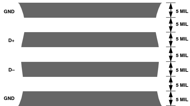
Figure 23. Typical Arrangement of Signal Tracks
