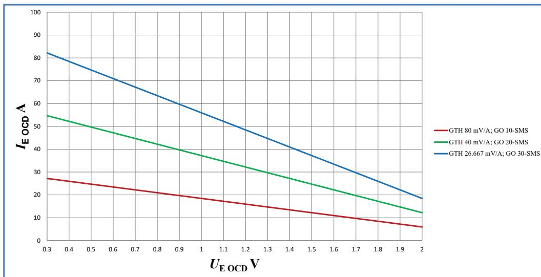
$$I_{E\text{ OCD}} = \frac{(V_{ref} - U_{E\text{ OCD}})}{G_{Th}} \times 1000 \quad U_{E\text{ OCD}} = \frac{R_E}{R_E + R_{ref}} \times V_{ref}$$
