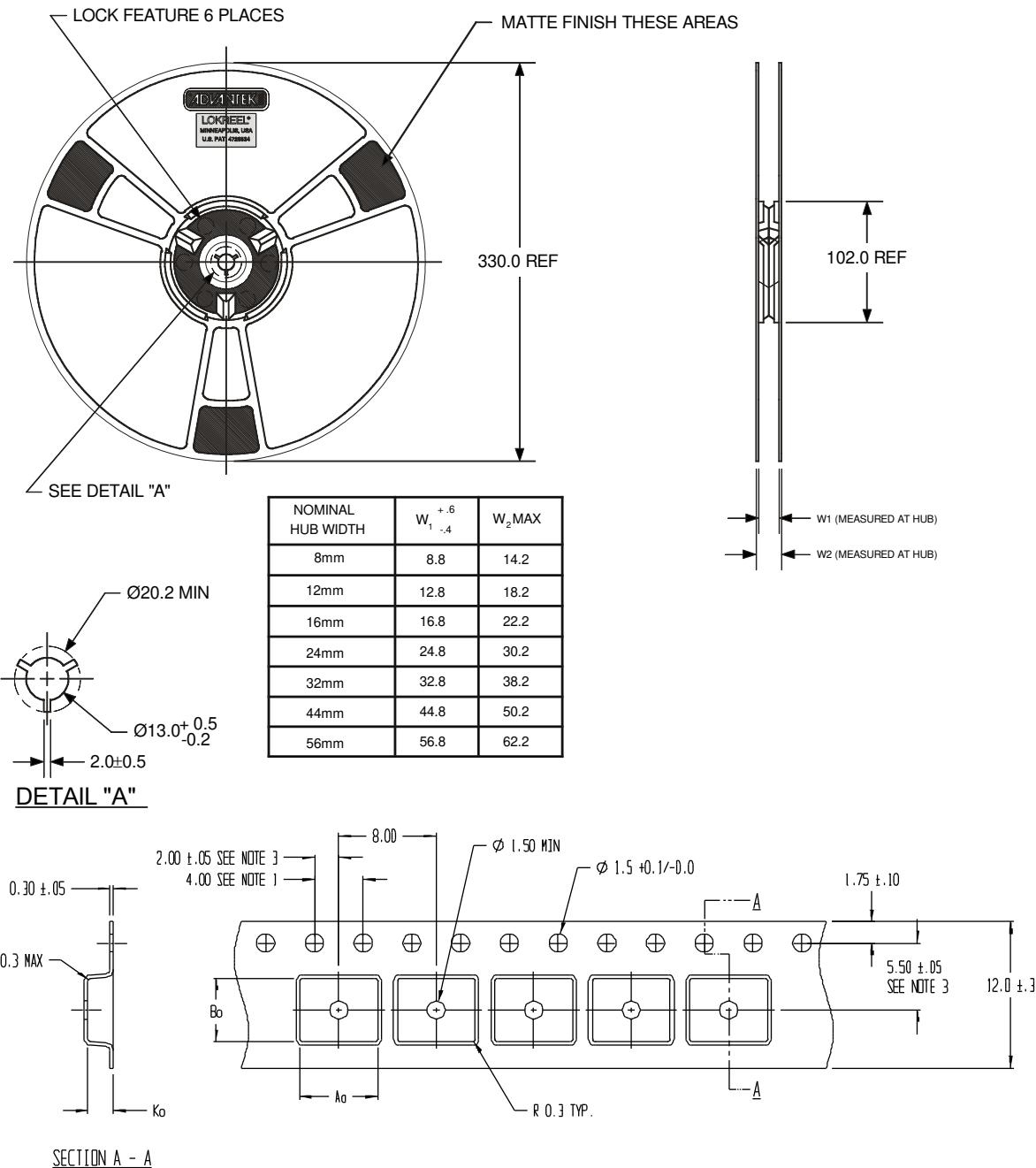
**Notes:** 1) 10 Sprocket hole pitch cumulative tolerance  $\pm 0.2$  mm
