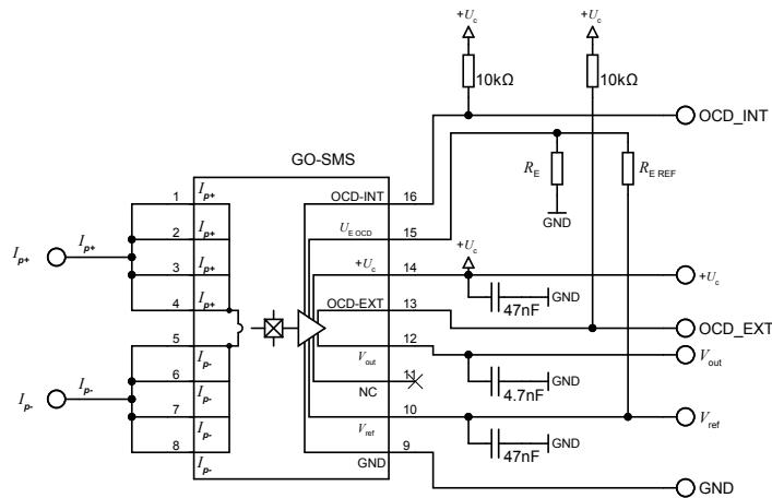
$I_{E\text{ OCD}}$ : External overcurrent detection (OCD threshold)
