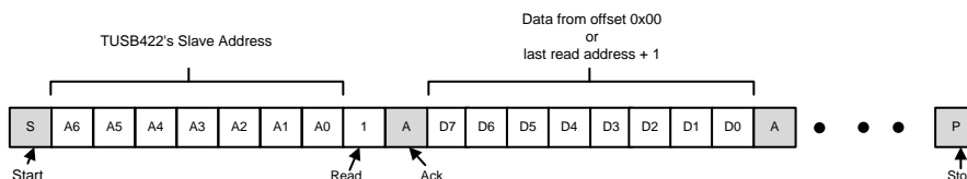
Figure 7. I2C Read Without Repeated Start
