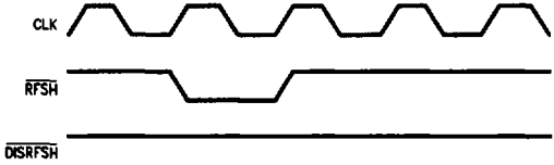
FIGURE 20a. Clearing the Refresh Address Counter
