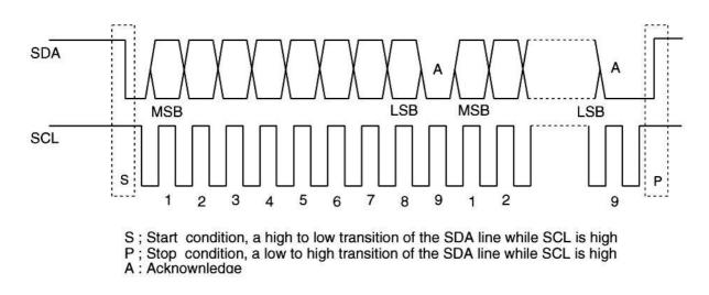
Every byte put on the SDA line must be 8-bits long . Each byte has to be followed by an acknowledge bit. Data is transferred with the most significant bit (MSB) first . The data on the SDA line must be stable during the HIGH period of the clock . The HIGH or LOW state of the data line can only change when the clock signal on the SCL line is LOW .
