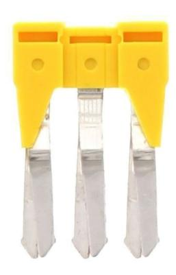
Insulated cross-connector, No. of poles: 3, Mounting type: Plug in, Width: 15 mm, Rated cross-section: 2.5 mm², Colour: Yellow
