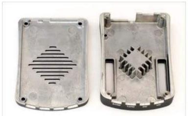
The ALU case is designed in a way that serves entirely as a big heat sink. On the interior part of the housing there is a large 16x16x12mm block which is directly connected to the FPGA of the STEMIab and in this way passes all the heat to the housing.
