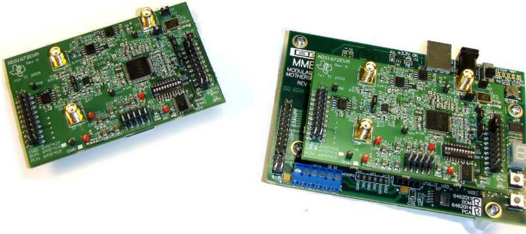
ADS1672EVM (Left) and ADS1672EVM-PDK (Right)
