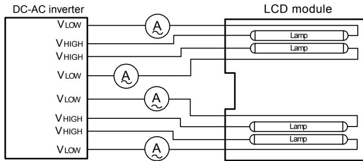
Connect the High Frequency Current Meter to the Low-Voltage (VLOW) si de.
