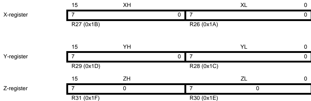
Figure 6-3. The X-, Y-, and Z-registers
