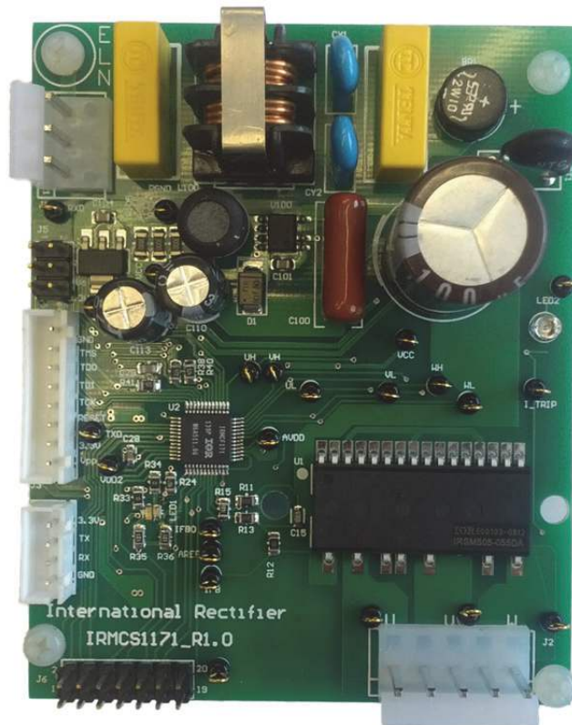
Figure 4: Reference design board featuring the \mu PM™-DIP module and the iMotion™ IRMCF171 digital control IC
