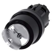
RONIS key-operated switch, 22 mm, round, plastic, lock number 455, with 2 keys, 2 switch positions O<I, momentary contact type, Actuating angle 45°, 10:30h/12h, key removal O, with laser labeling, lower case
