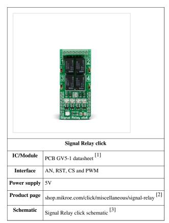
**Signal Relay click** carries four ultra-small GV5-1 PCB relays from Omron and runs on a 5V power supply. The click communicates with the target MCU over the following mikroBUS pins: AN, RST, CS and PWM.
