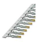
Crimp contact, Socket, rolled, Taped articles, number of pieces per reel: 10000, contact diameter: 1 mm, crimp range:  $0.22 \text{ mm}^2 \dots 0.56 \text{ mm}^2$ , Item is lead-free in accordance with RoHS II without Exemption 6c (Pb <0.1%)
