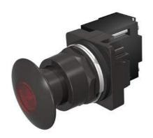
30mm BlackMax, Epoxy Coated Corrosion Resistant Complete Metal Unit Illuminated Push-Pull Operator Transformer type, 120V AC LED Lamp Mushroom Head Cap Small 1 3/4" (44.5 mm) Metal, Black with Red Lens 3 Position Momentary UL Listed, CSA Certified NEMA 1,3,3R,4,4X,12,13 & Automotive Standards
