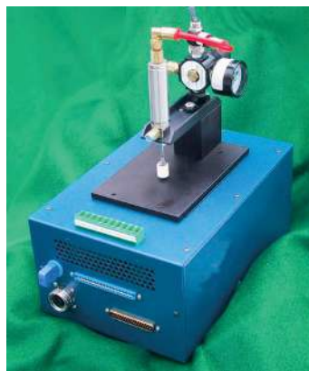
Figure 3-9: \theta_{JC} Measurement Setup
