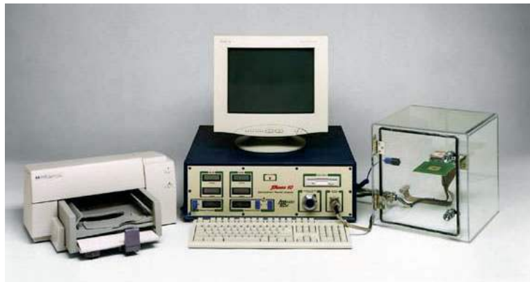
Figure 3-10: \theta_{JA} Measurement Setup
