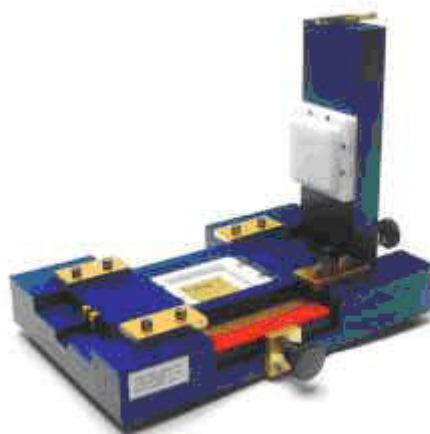
Figure 4-1: Altair BGA Fixture Used for TDR Measurement
