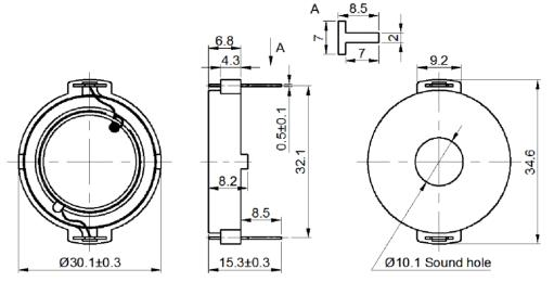
General tolerance = ±0.5 mm and all measurements in mm unless otherwise noted.
