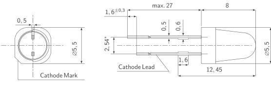
all dimensions in mm. Tolerance  $\pm 0,\,1$  except given ones  $^{\ast}$  at the bottom of the LED
