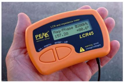
Continuous measurements with hold function
